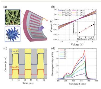
**Fig. 3** (a) Schematic illustration of the UV photodetector fabricated from the ZnO-MWCNT hybrid paper. (b) Typical *I–V* characteristics of the UV photodetector measured with varying light intensity. The inset shows the power-dependent photocurrent of the device at -5 V bias under UV illumination. (c) Transient response and (d) photoresponsivity spectra of the UV photodetector.
