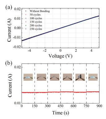
**Fig. 5** (a) I-V curves of the flexible hybrid photodetector under UV illumination without bending and after 50, 100, 150, 200, and 250 cycles of bending. (b) The I-t curve of the flexible hybrid photodetector when bent with different curvatures under a bias voltage of -5.0 V. The insets are corresponding photographs of the device under the different bending states.
