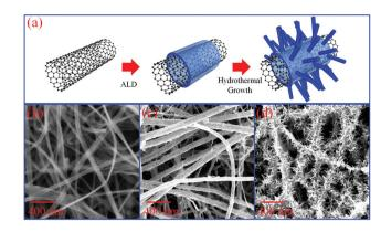
**Fig. 1** (a) Schematic illustration showing the fabrication process of the flexible thorn-like ZnO-MWCNT hybrid paper. High resolution scanning electron microscopy (SEM) images of the sample in each fabrication step: (b) bare MWCNT paper, (c) MWCNT paper covered by a thin and uniform ZnO seed layer using ALD, and (d) thorn-like ZnO-MWCNT hybrid paper formed after hydrothermal growth.
